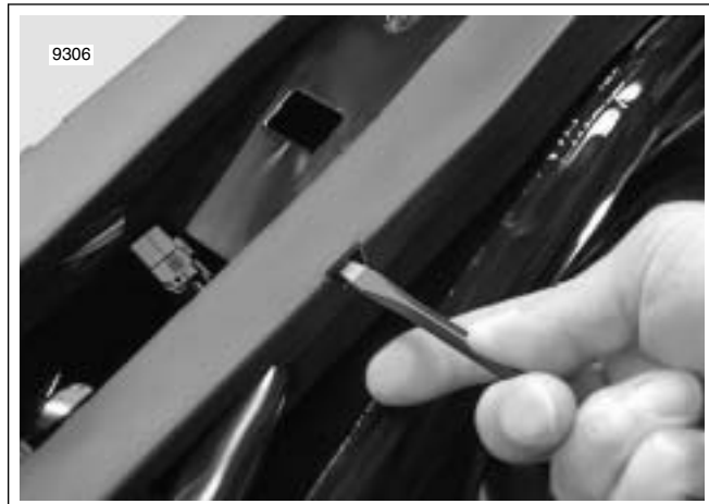
Figure 8-150. Release Catches From Cover
