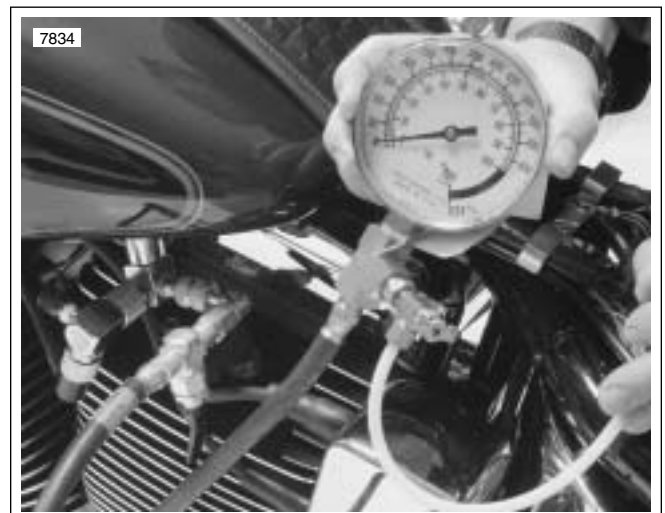
Figure 5-34. Fuel Pressure Gauge Installed (Typical)
