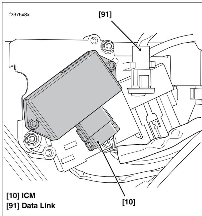
Figure 8-48. Under Right Side Cover (Carbureted)
