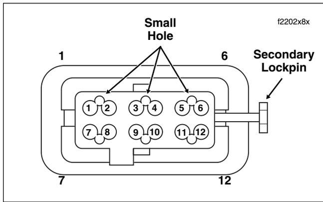
**Figure 8-27. Mating End of Connector**
