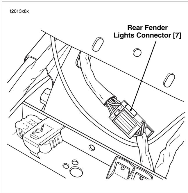
Figure 8-49. Rear Fender (Under Seat)
