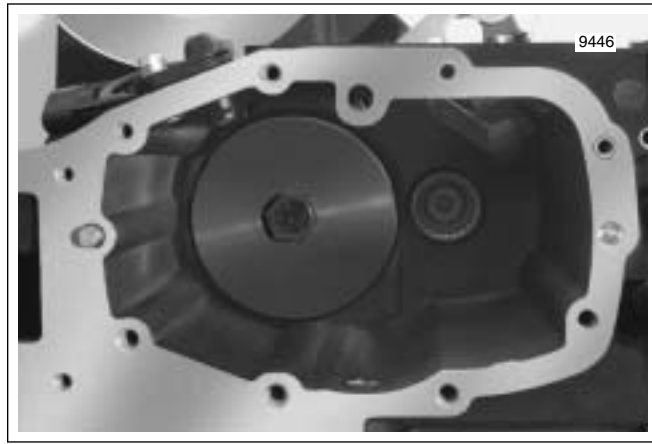
Figure 7-36. Main Drive Gear Installation (Right Side)
