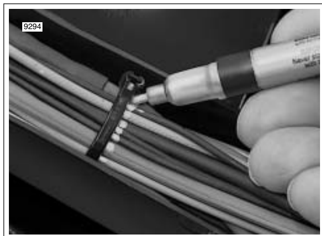
Figure 8-151. Mark Location of Cable Straps
