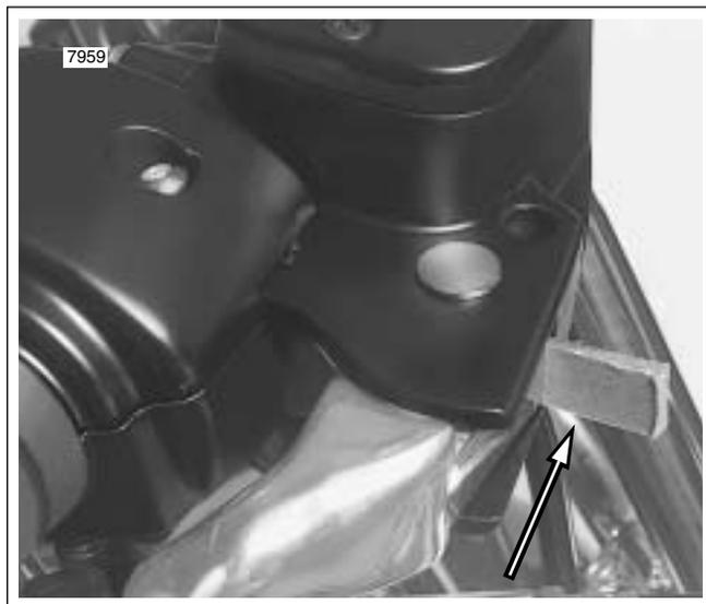
Figure 2-43. Install Cardboard Insert
