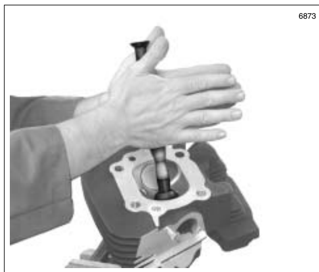
Figure 3-25. Oscillate Valve Lapping Tool to Create Contact Area
