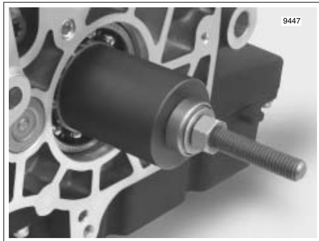
Figure 7-37. Main Drive Gear Installation (Left Side)
