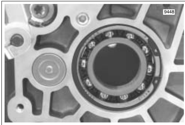
Figure 7-38. Install Retaining Ring With Gap Facing Rear
