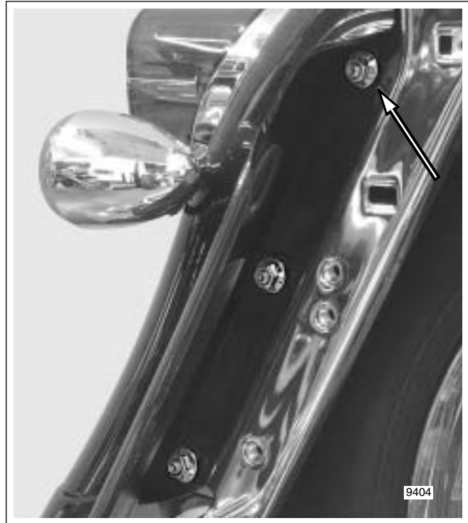
Figure 2-198. Remove Flange Nuts
