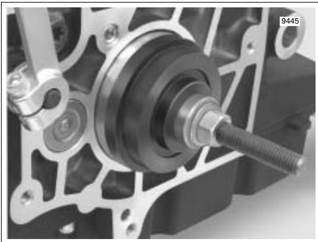
Figure 7-35. Main Drive Gear Bearing Installation (Left Side)
