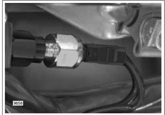
Figure 8-114. Rear Stoplight Switch
