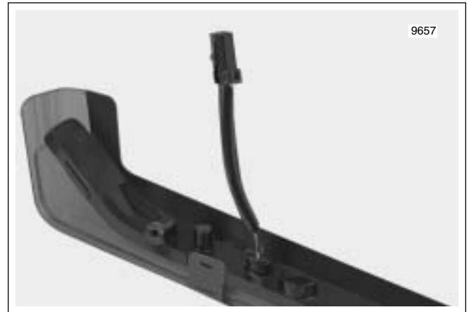
Figure 2-155. Side Marker Lights Assembly (FLHTCU)
