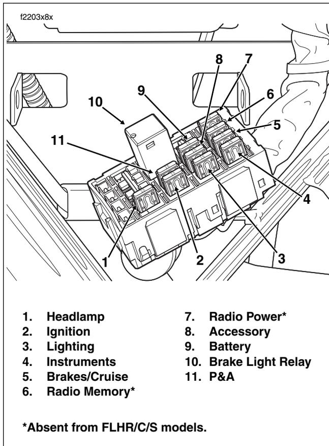
Figure 8-44. Fuse Blocks - FLHX, FLHTC/U, FLTR (Under Left Side Cover)
