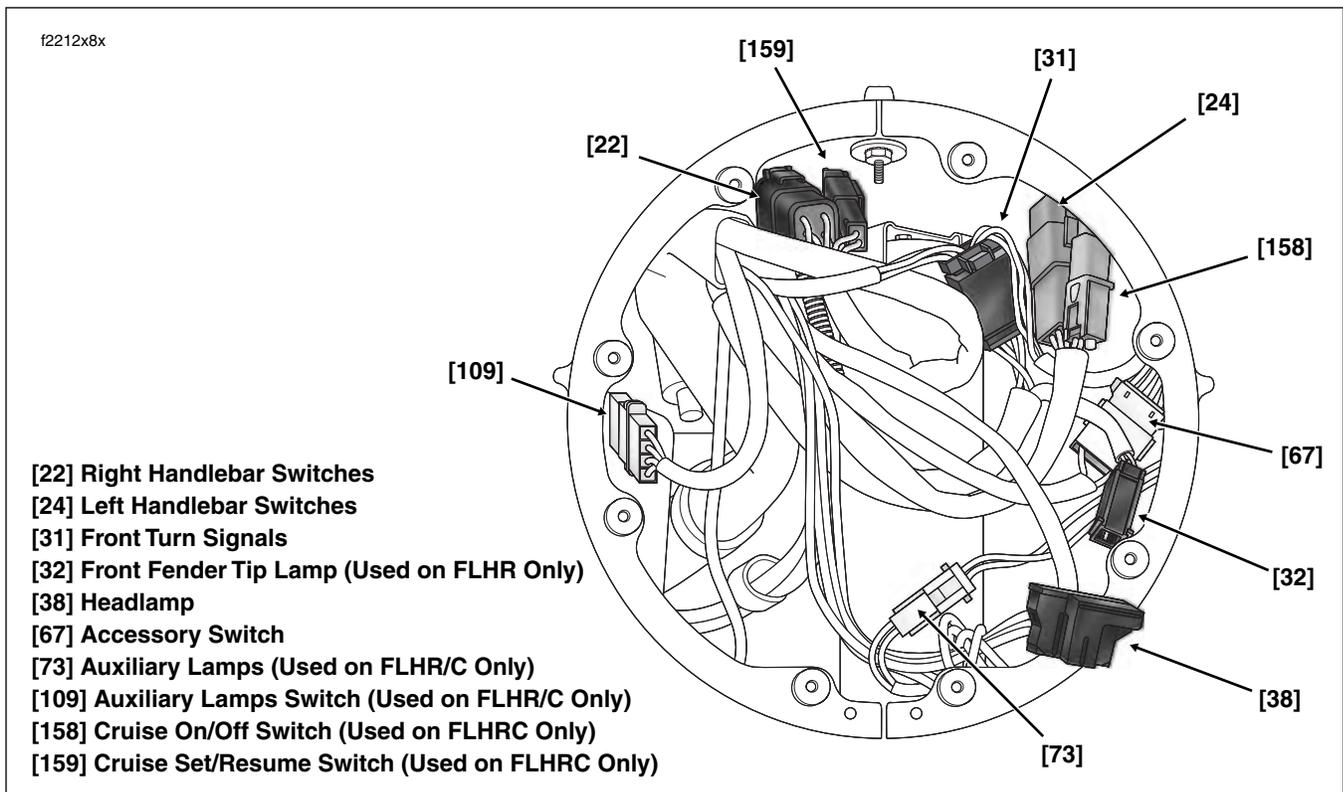
Figure 8-55. Headlamp Nacelle Connectors (FLHR/C/S)
