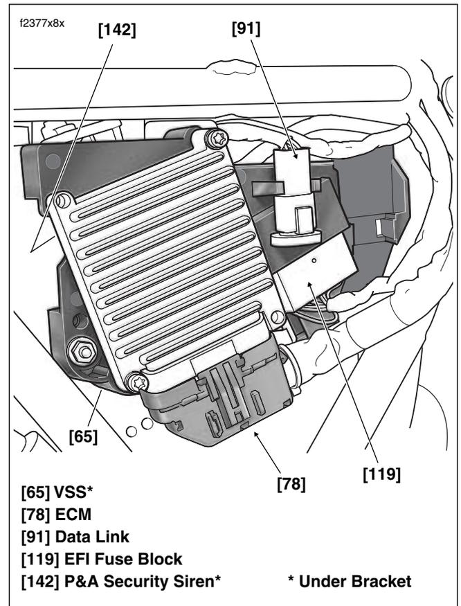
Figure 8-45. Under Right Side Cover (Fuel Injected)
