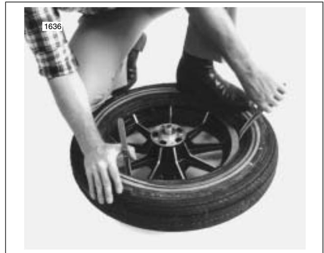
Figure 2-34. Starting Second Bead on Rim
