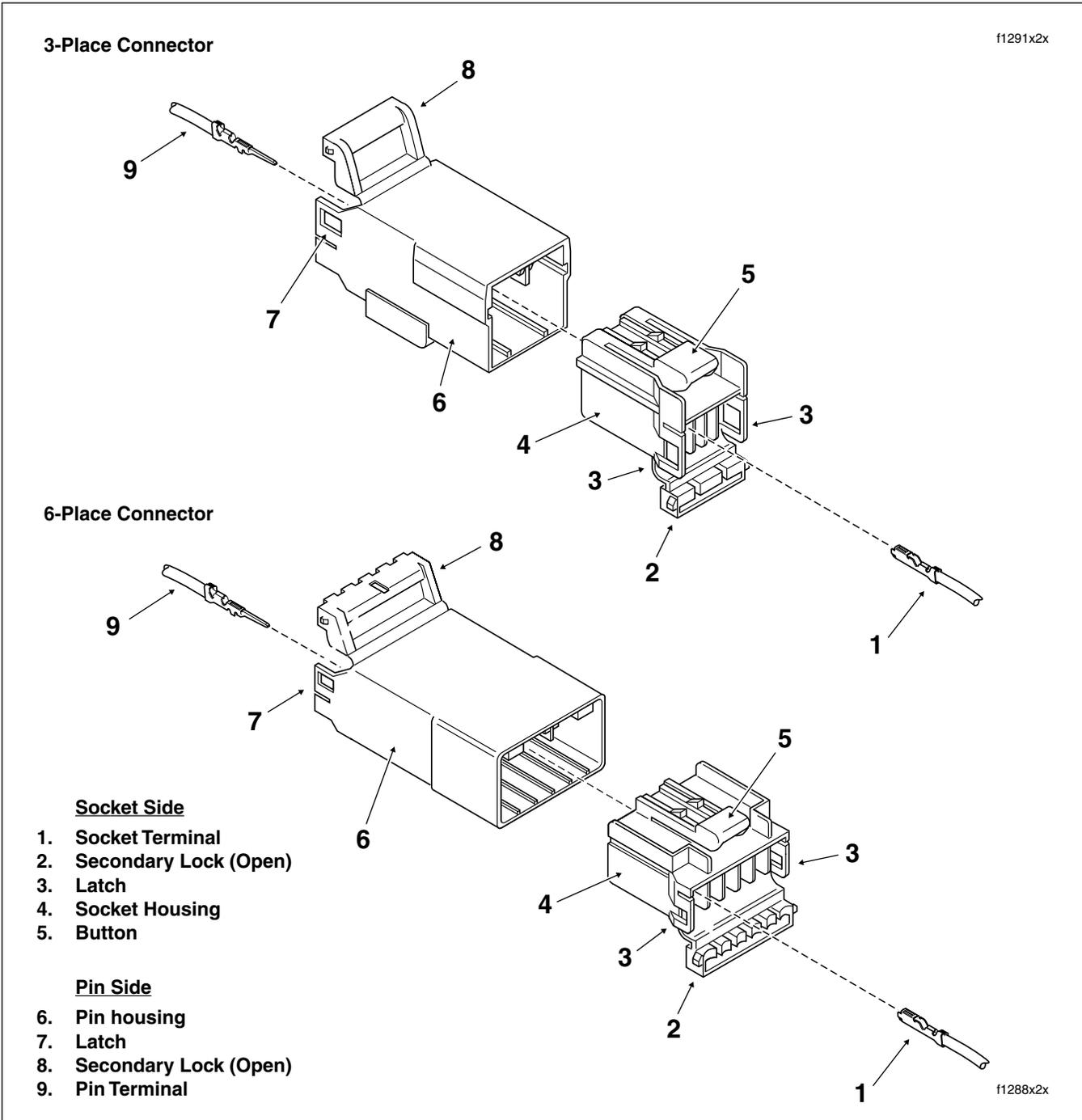
Figure 8-14. 3-Place and 6-Place Multilock Connectors
