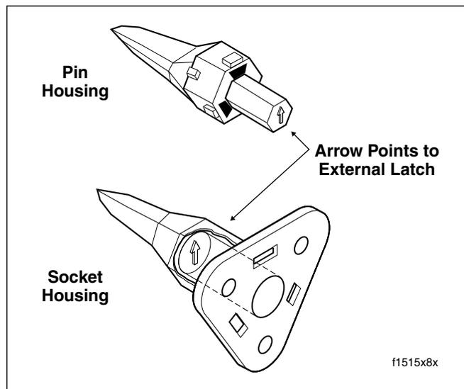
Figure 8-4. 3-Place Locking Wedge Orientation
