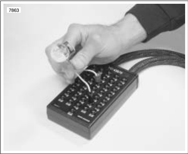
Figure 5-66. Ignition Coil Circuit Test
