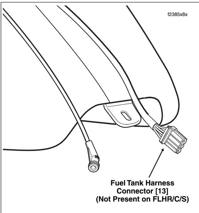
Figure 8-47. Rear of Fuel Tank (Under Seat)
