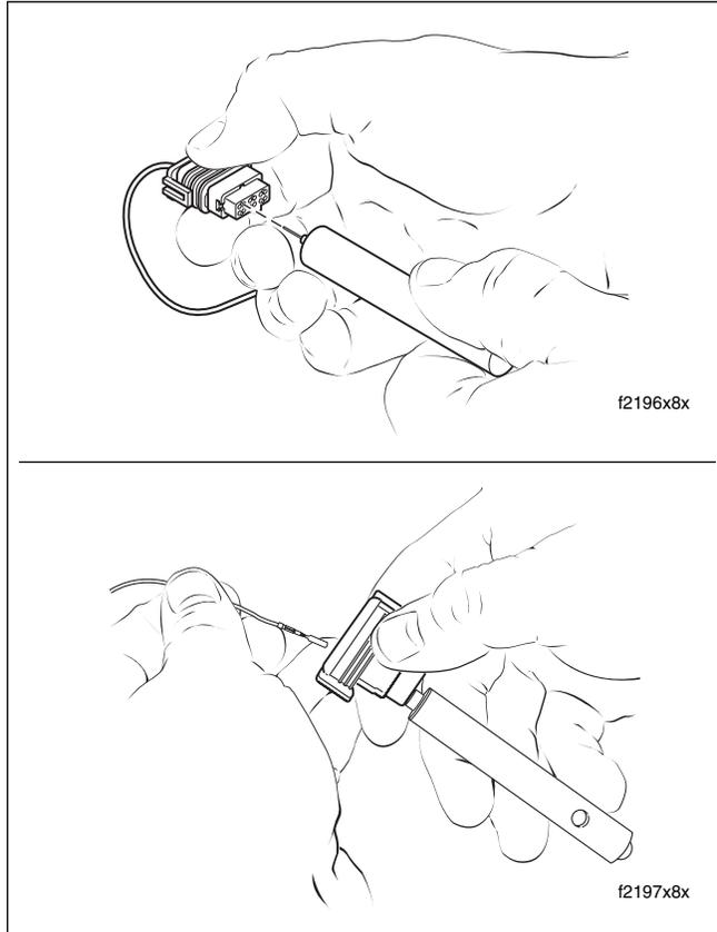
**Figure 8-28. Insert Tool and Remove Terminal**
