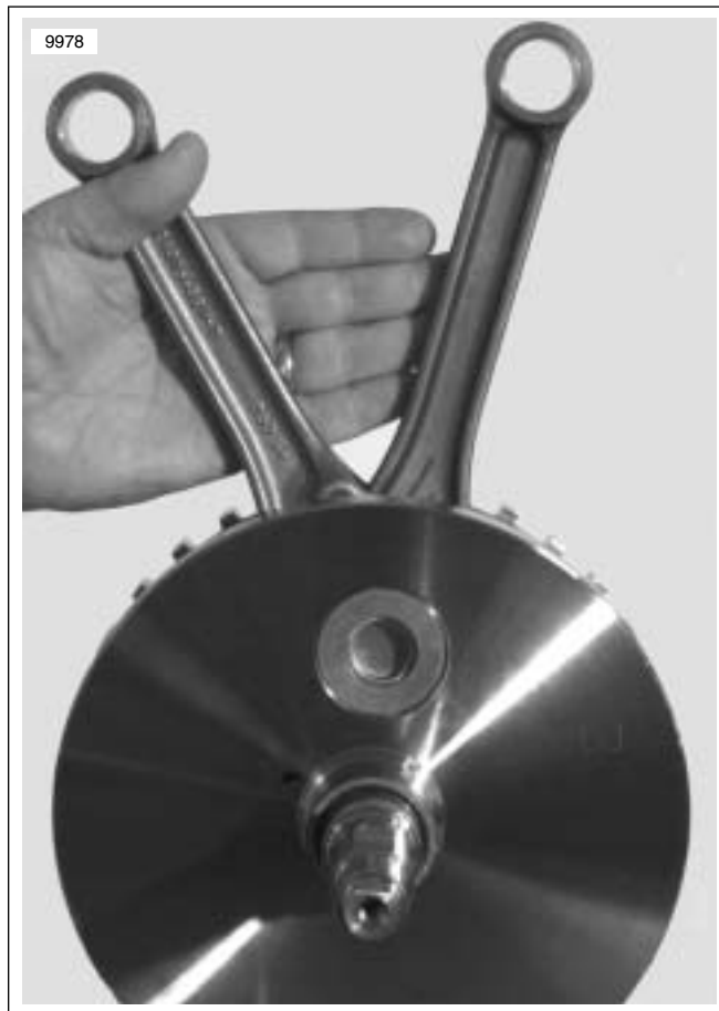
Figure 3-35. FLHTCUSE Flywheel/Connecting Rod Assembly
