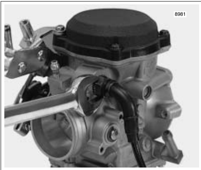
Figure 4-5. Remove Enrichener Cable
