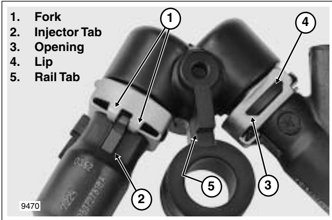
Figure 9-30. Install Spring Clips
