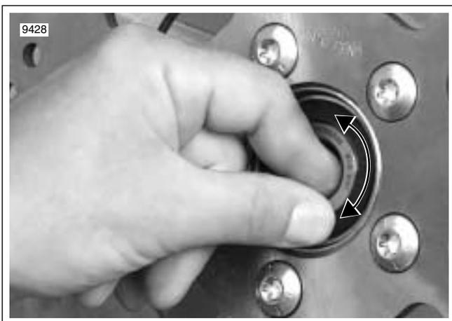
Figure 2-2. Inspect Wheel Bearings
