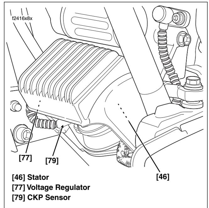
Figure 8-51. Voltage Regulator (Left Side View)
