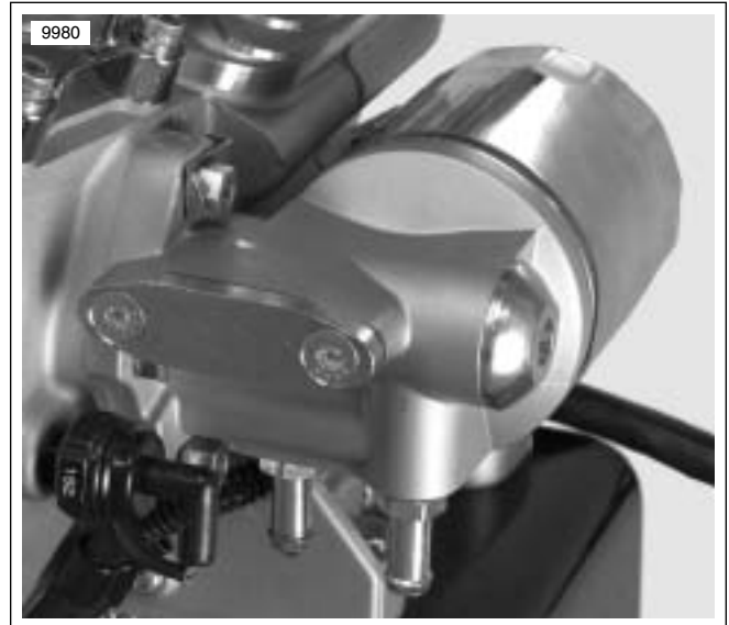
Figure 3-50. Oil Filter Mount (engine removed from frame)
