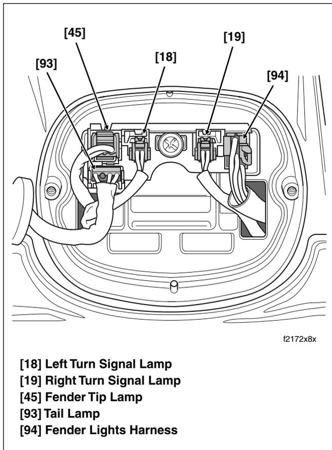
Figure 8-50. Rear Fender Lights Assembly
