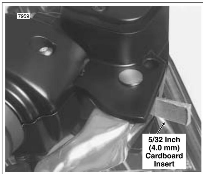
**Figure 8-87. Install Cardboard Insert**
