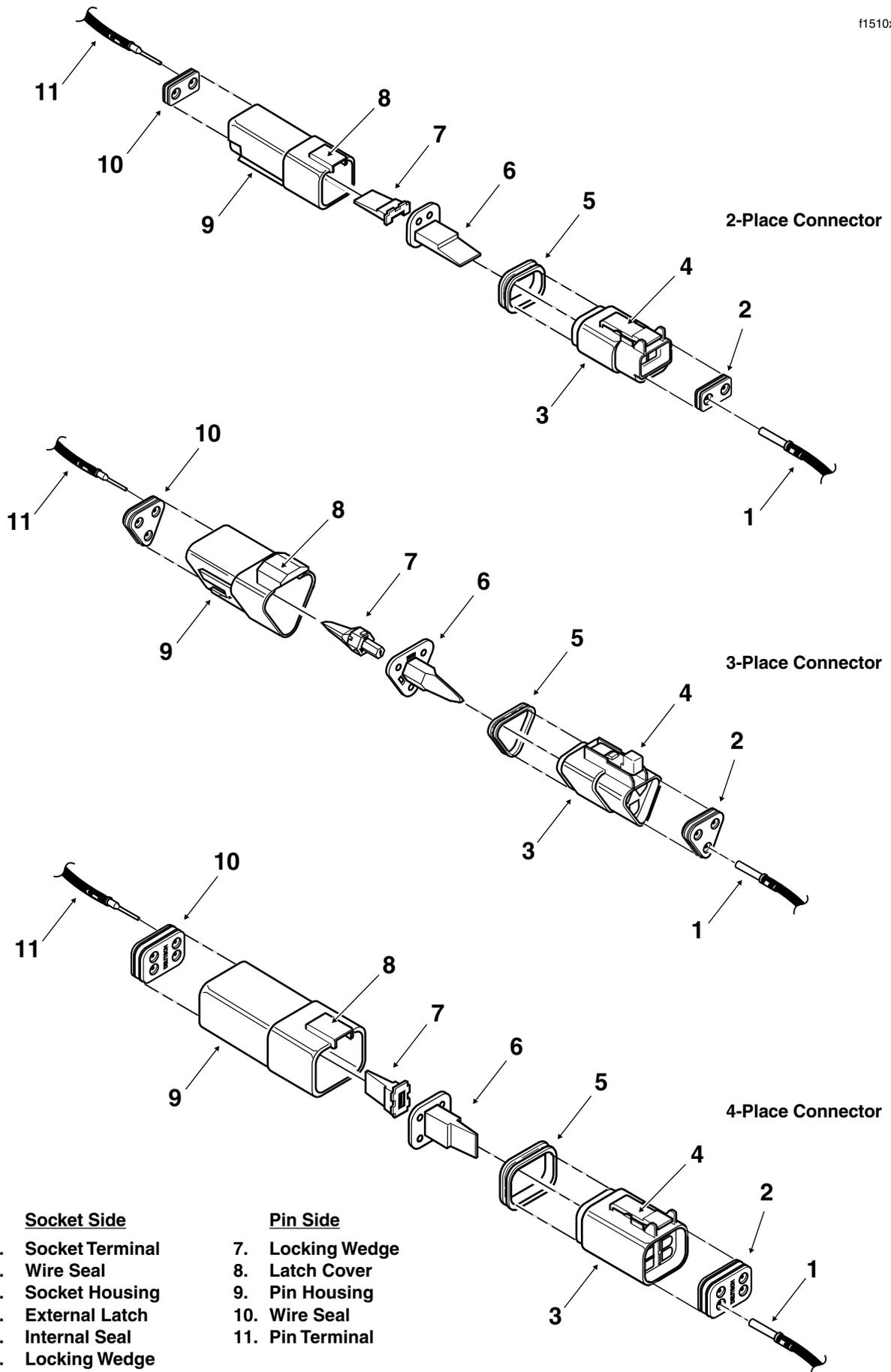
Figure 8-5. 2-Place, 3-Place and 4-Place Deutsch Connectors
