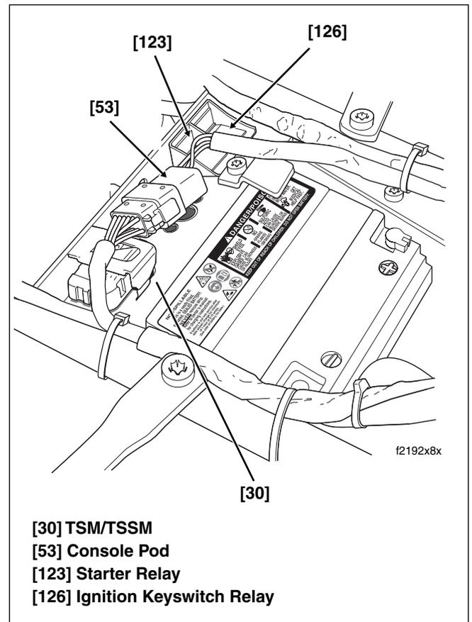
Figure 8-52. Electrical Connectors/Relays (Under Seat)
