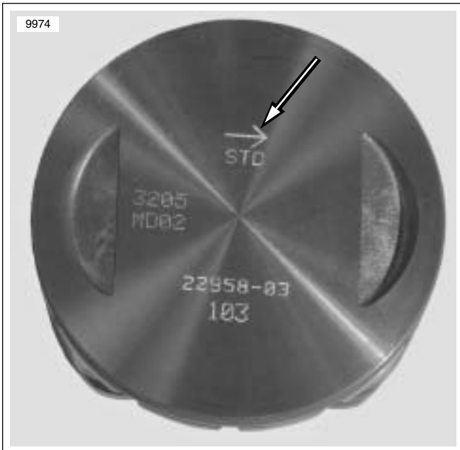
Figure 3-32. FLHTCUSE Piston Orientation Arrow (arrow points to front of engine)
