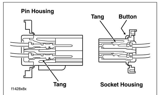
Figure 8-12. Tang Location (Cross Sectional View)
