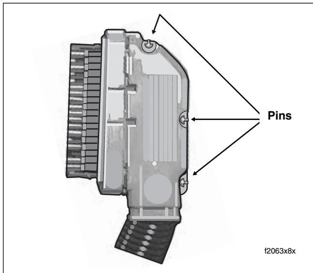
Figure 8-34. Separate Halves of Socket Housing
