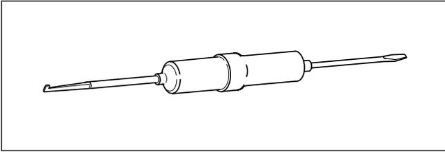
**Figure 8-6. Deutsch Connector Pick Tool
