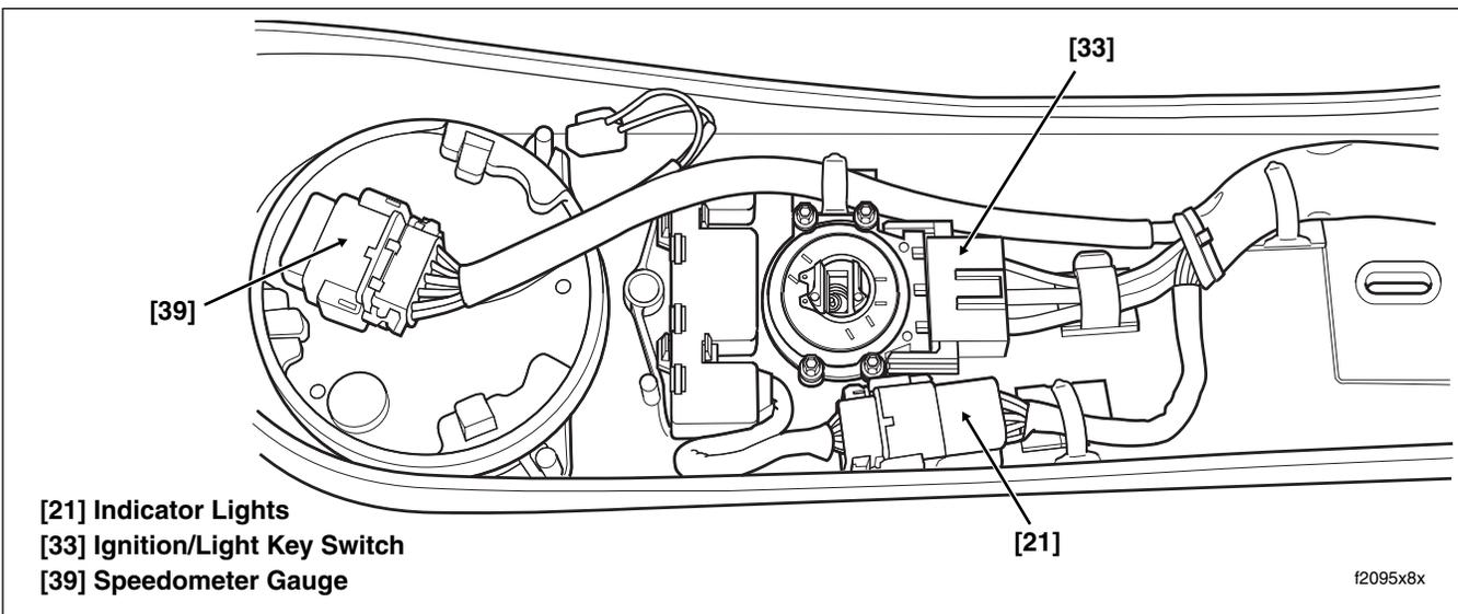
Figure 8-56. Instrument Console Connectors (FLHR/C)
