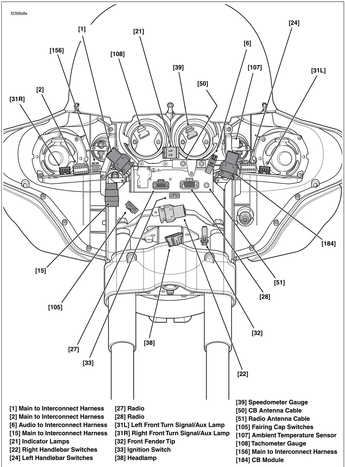
Figure 8-41. Inner Fairing Connectors (FLHX, FLHT/C/U)
