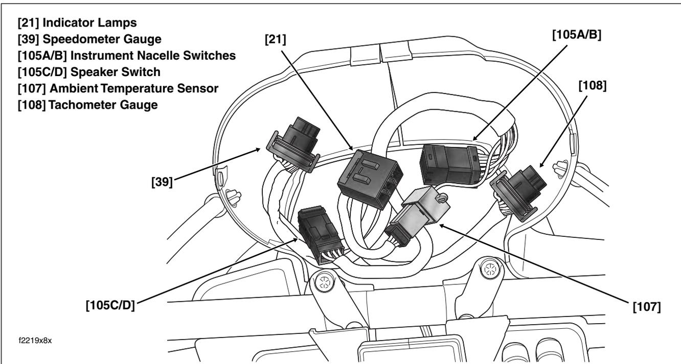
Figure 8-53. Instrument Nacelle Connectors (FLTR)
