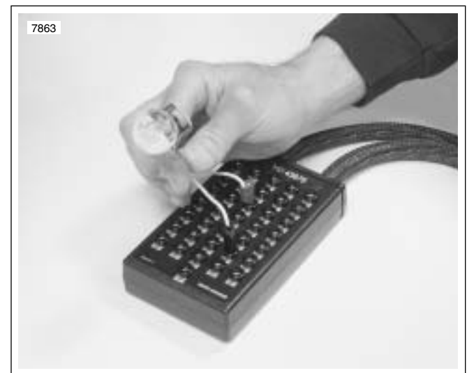
Figure 5-17. Ignition Coil Circuit Test
