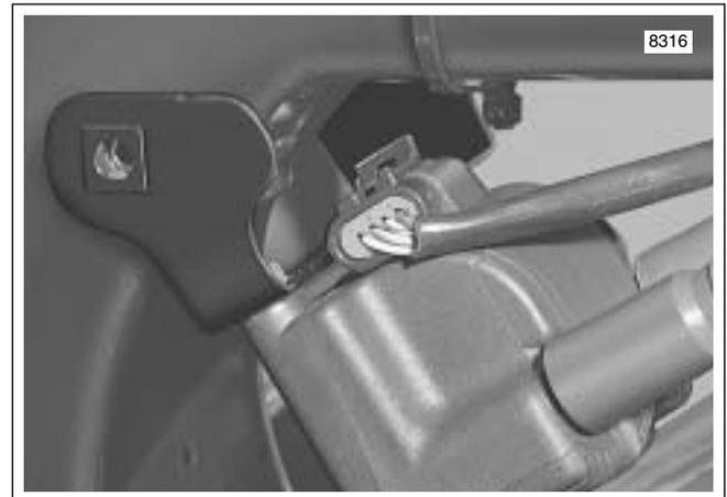
Figure 3-11. Remove Ignition Coil Bracket
