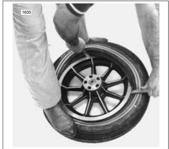
Figure 2-33. Starting Bead on Rim
