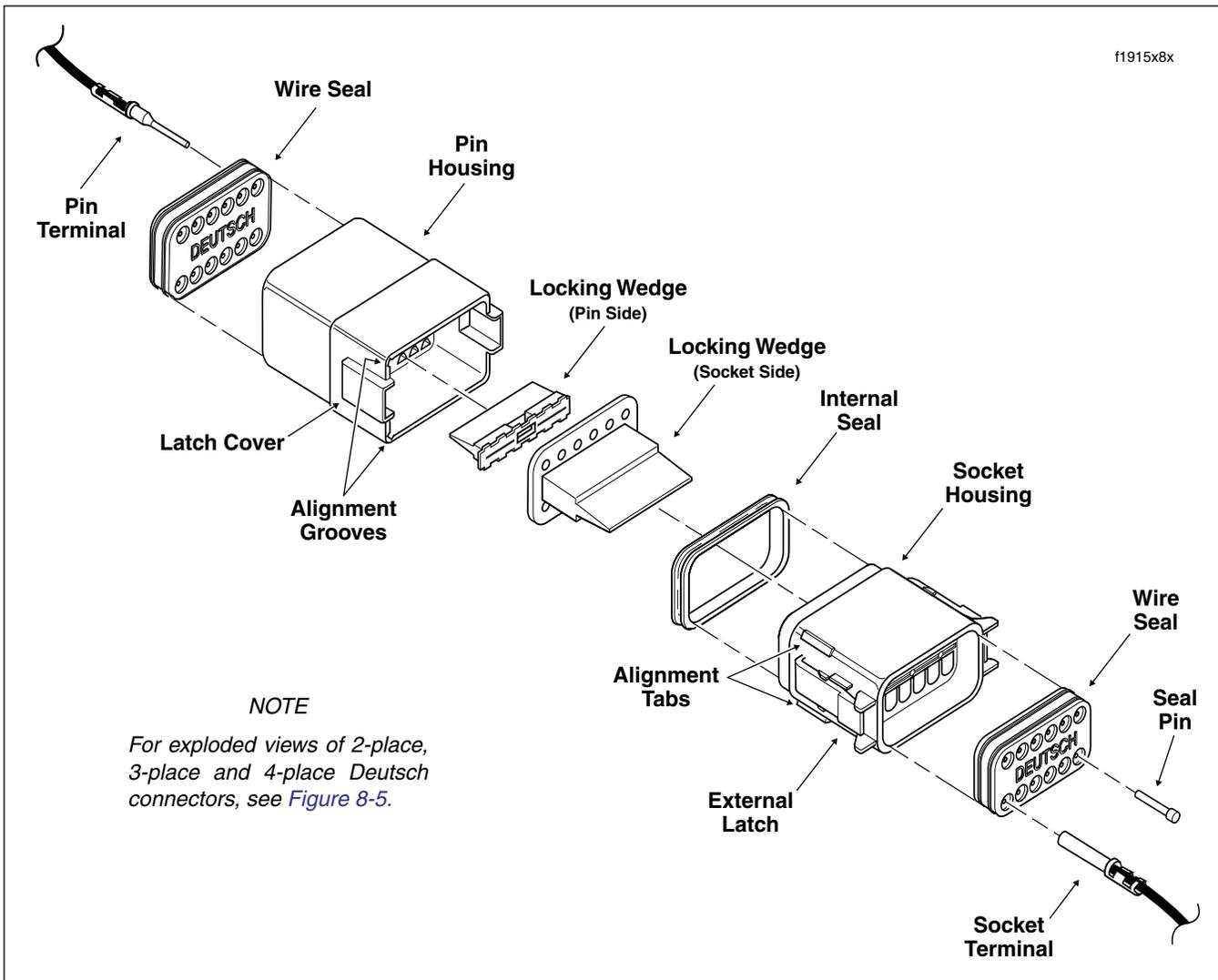
Figure 8-3. 12-Place Deutsch Connector (Exploded View)
